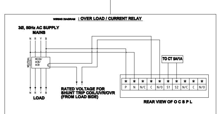
NOTE 1: IT IS DESIRABLE TO DERIVE AUXILIARY VOLTAGES/SUPPLY USING SEPERATE AUXILIARY TRANSFORMER FROM MAINS, OF SUITABLE RATING.
